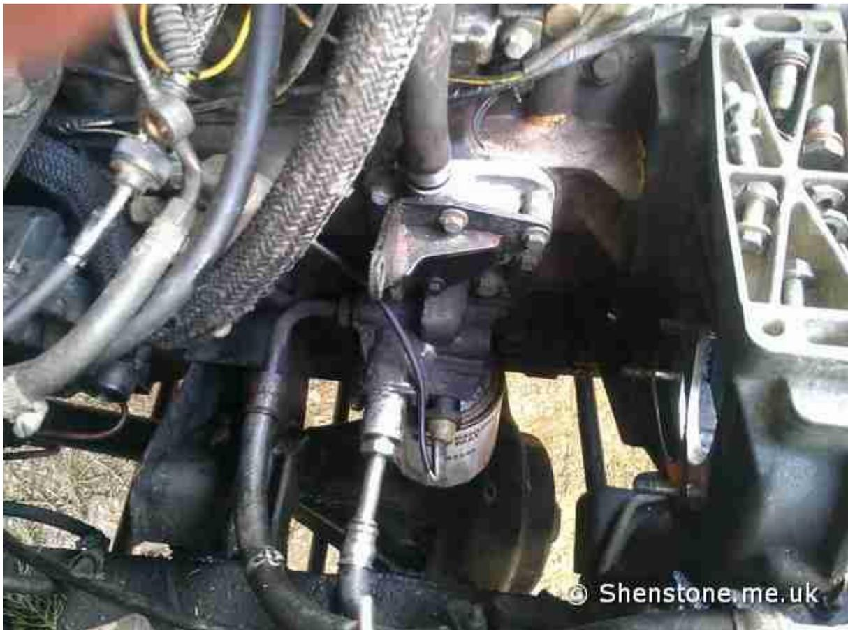
But in doing that, it was noted that the tensioner pulley for the fan belt was seized and that means a new one so that's off as well, a nice and simple job of removing the single bolt that holds it in and it wasn't even seized or anything and came off really easily
