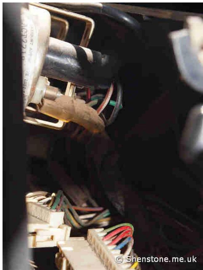
We had been told not to connect these from the back of the speedo/fuel gauge and temperature gauge bit to go behind them and find another multiconnector, which is the black one in the picture below. It
