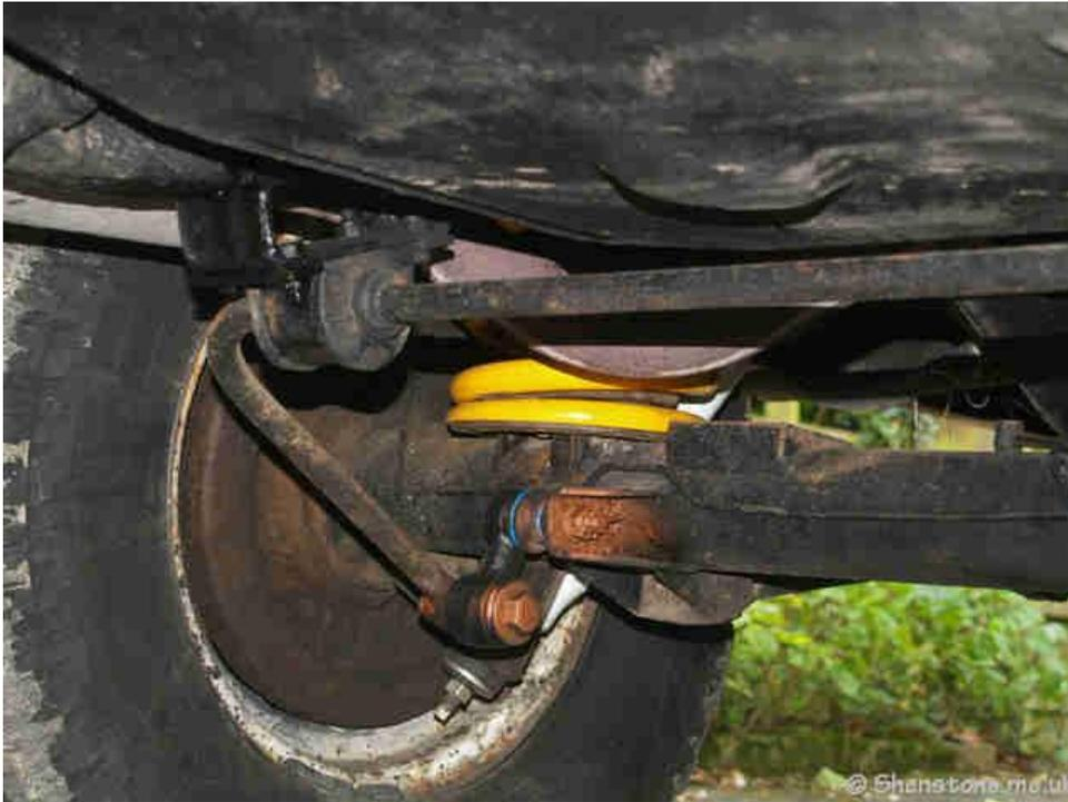
And in this slightly wider view you can see the complete anti roll bar running across the fuel tank
