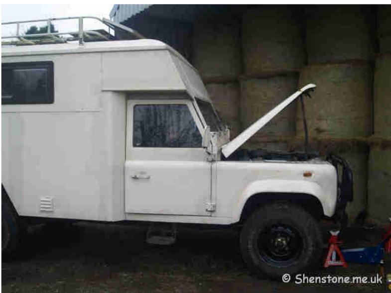
First the wheels came off for access and Katy was resting on the new axle stands I bought recently. This allowed the wheels to drop and take the compression out of the springs, but you need to be careful not to allow them to drop too far or the brake lines will be damaged, so I kept Steve's trolley jack under the axle for control and adjustment.
