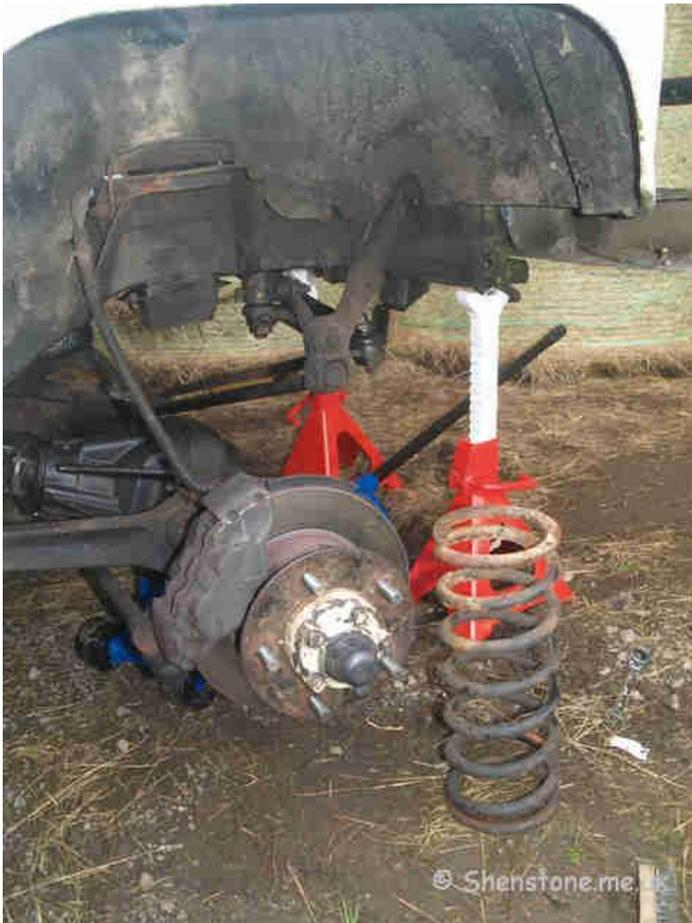
Before rebuild began I took the opportunity to clean a few things up and put some liquid grease on the brake pipes and into the corners behind the springs that had not been east to get to when I was doing the waxolyling
