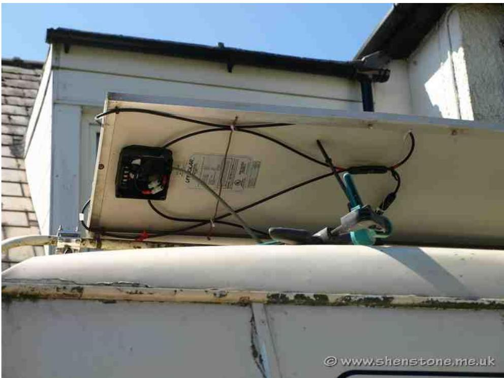
From this last picture you can see the old frame which was bolted to the roof-rack and to the blue light bracket on the roof. Once it was connected, I took the cardboard I had temporarily put over the
