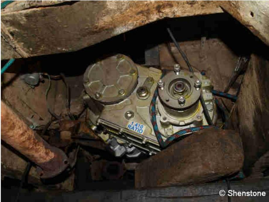
When you put it back it is useful to have it in difflock so you can rotate either of the propshaft takeoff's in order to get the spline from the gearbox lining up. This was a key bit of knowledge from Steve, and something achieved with a pair of molegrips on the selector.
