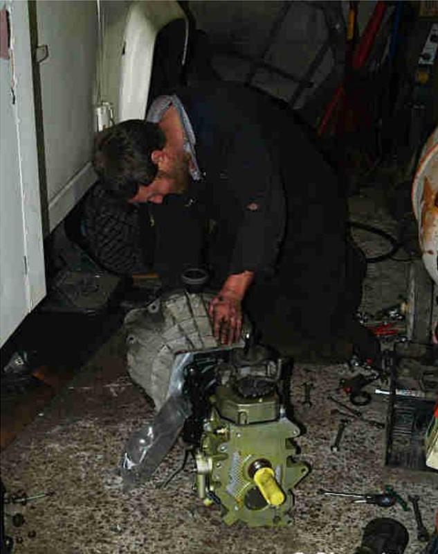
Steve fitting the clutch fork into the newly refitted bell housing
