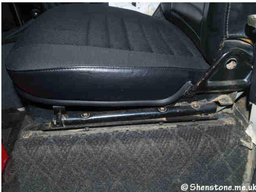
Quickly remove the bases for better access and remove the 4 bolts at each corner (you can see 2 here at the far left and right).
