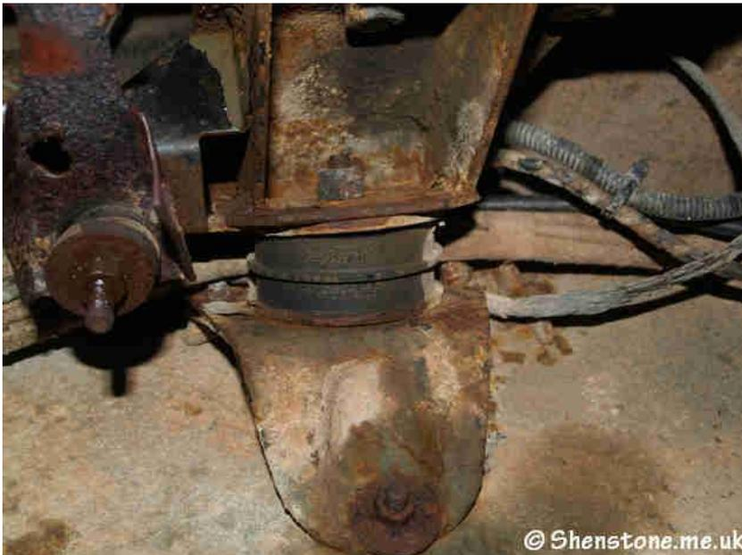
Back up on top I had to disconnect some more wire's I found which are just twisted together as a connection and then attach a safety rope to the transfer box which was lashed to a crowbar which was placed across the 2 front seat bases, and another in my hand so I could maneuver it.
