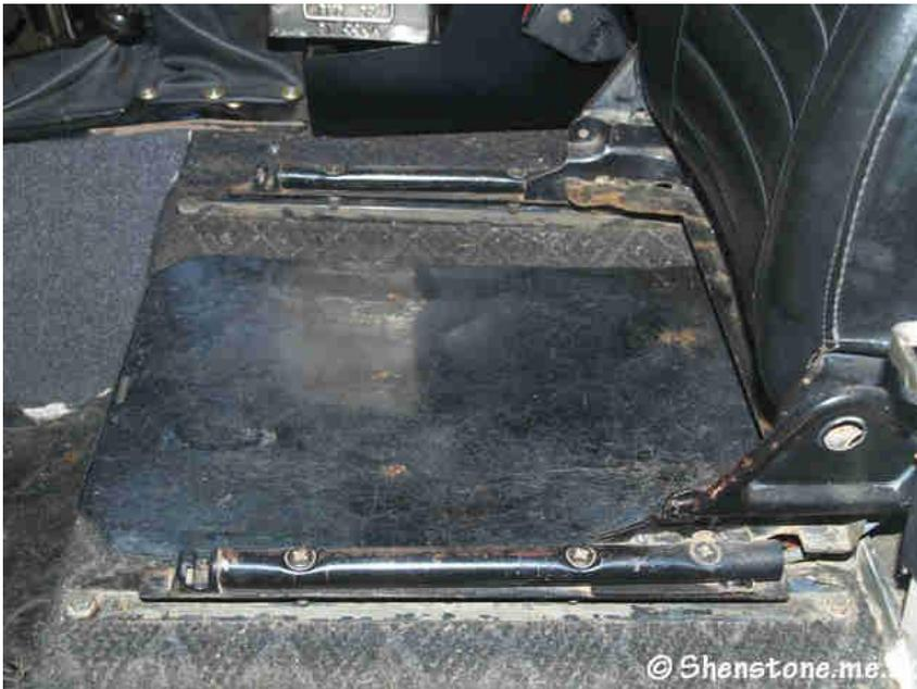
Then I hit a snag - I was not able to get the rear bolt near the center because of the broken seat back so I removed the seat from the bars by removing the 6 bolts at that point (I left the others in place to stop everything moving whilst I was doing that which is why they are visible in this picture).
