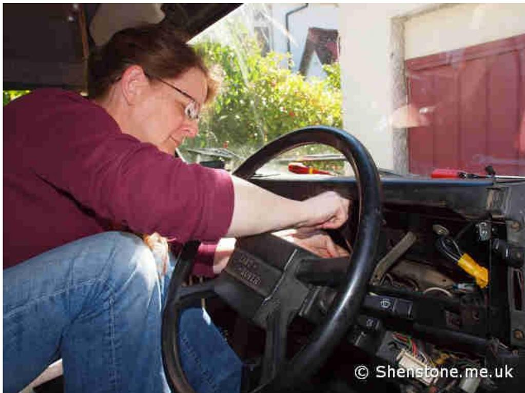
The Speedo cable plugged in as easy as it came out so that was easy and we upgraded the bulbs to new LED's as well, and the result. ... clean instruments that work and do not rattle around when you are driving and I can see at night
