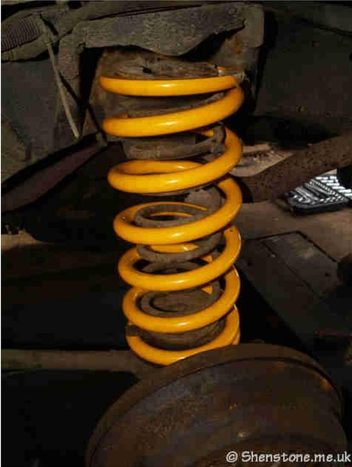
Finally reattach the shock absorbers, put the wheel on, reattach the Anti Roll bar linkage the and all was done for the day.
