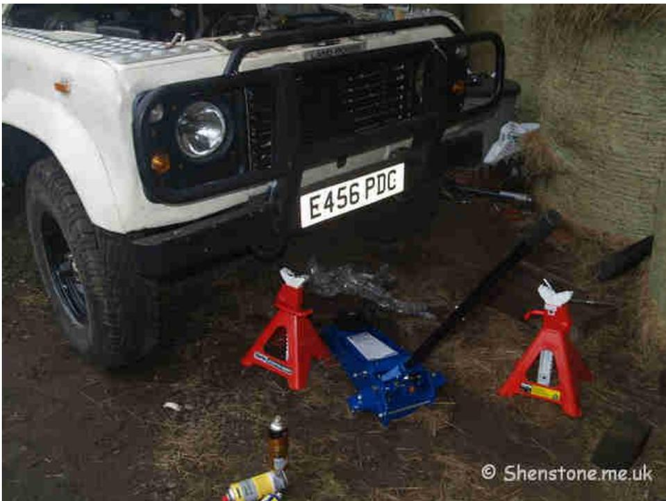
It was then then a relatively simple job of unscrewing the bottom of the shock absorber (damper) which needs the shock to be held in place or it just turns. A flexible strap is a great tool for this and the job was quickly done.
