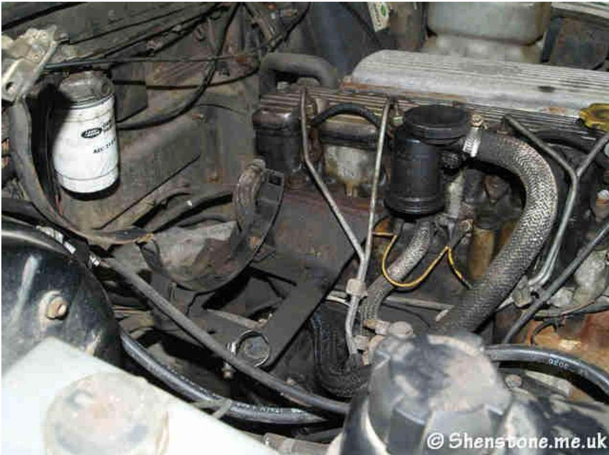
I'd been applying "shock and unlock" , and WD40 liberally to bolts for a few days leading up to this work to ensure it had time to fully lubricate the threads and give us a good chance of removing them rather than cutting them. it really paid off when it came to removing the front cross member as you can see from below where all the bolts came out easily leaving us just needing to spread the chassis a little with one of Steve's hydraulic jacks in order to lower it out
