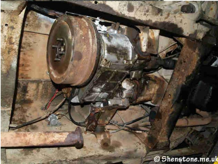
The next step was to remove a section of exhaust that was in the way and then remove one of the engine mounting brackets (which look a bit tired as you can see so we're replacing them), we then added a bottle jack to support the main gearbox so we could loosen off the other bracket and we were finally getting close to being able to get at least the Transfer box out.
