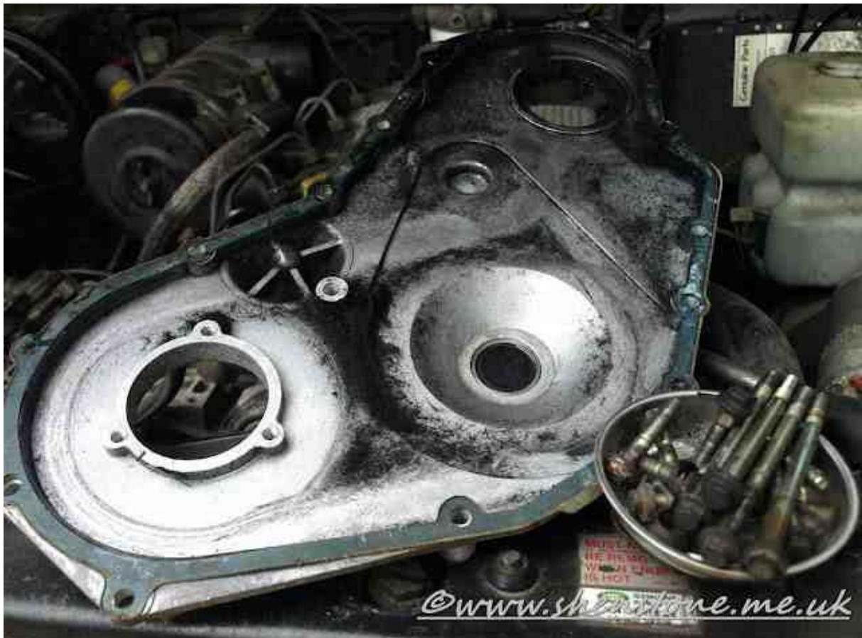
Whilst some of the teeth were still in place on the belt, others had been stripped off and had been transformed into all the fluff that you can see on the inside of the case in the picture above, and between the pulleys in the picture below
