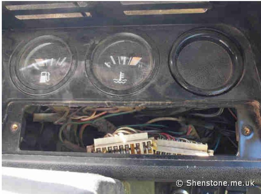
Then we undid the screws on the side of the binnacle (only one was actually holding it in) and we could pull it carefully and see the wires.
