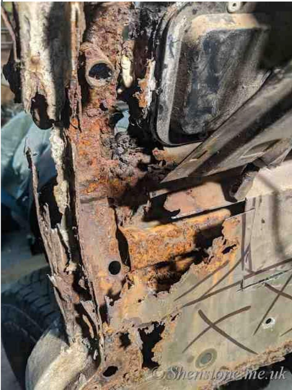
It's actually a bit better than it looks because some of that is just surface rust and can be treated, but we will be replacing those bits with air instead of metal.
