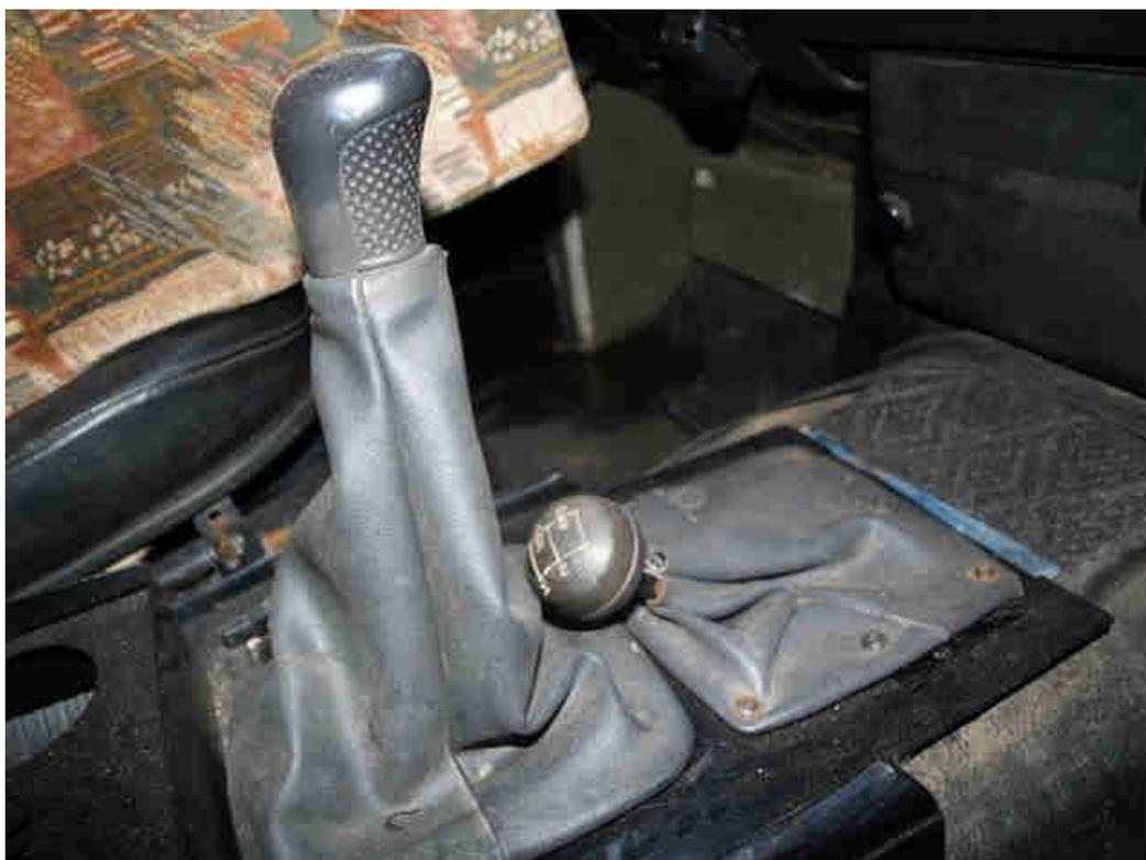
And the layout of the shifter is that of an R380 5 Speed box, which replaced the LT77 fitted from approx 1994 to 2006
