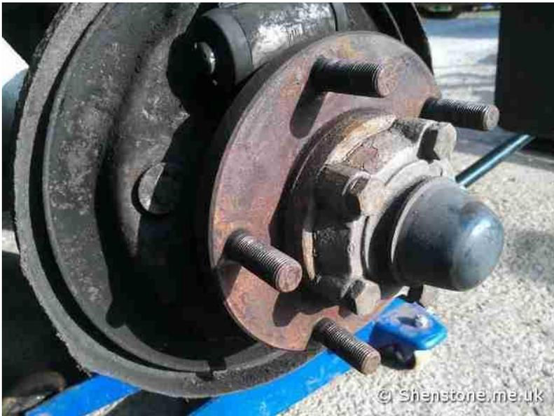
And you can see the corroded adjusters in the wheel - everything felt a bit unmoving or smoothed off so it had to be cut-off
