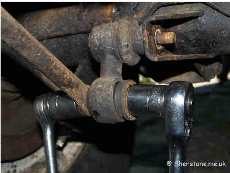
Removing the Anti Roll bar from the linkage with 2 sockets
