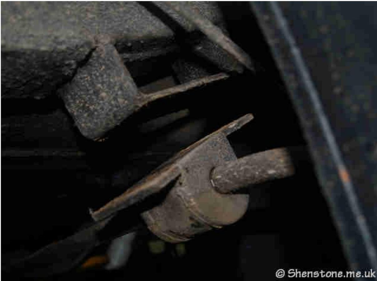
Next there was some adjustment as the new bars are narrower across than the old ones so the linkages needed turning around to fit. As I had fitted new ones [recently](#) with new polybushes these were not being replaced. it was a simple case of knocking them out...
