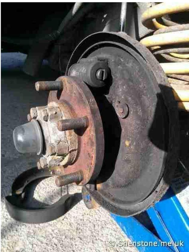
Then we hit the problem the kit provided did not seem to fit as the bolts in the front hit the brake pads. There seemed to be no sensible combination of the washers that could be made to fit with the adjuster so we made up a new next of washers that got the cam in the right place
