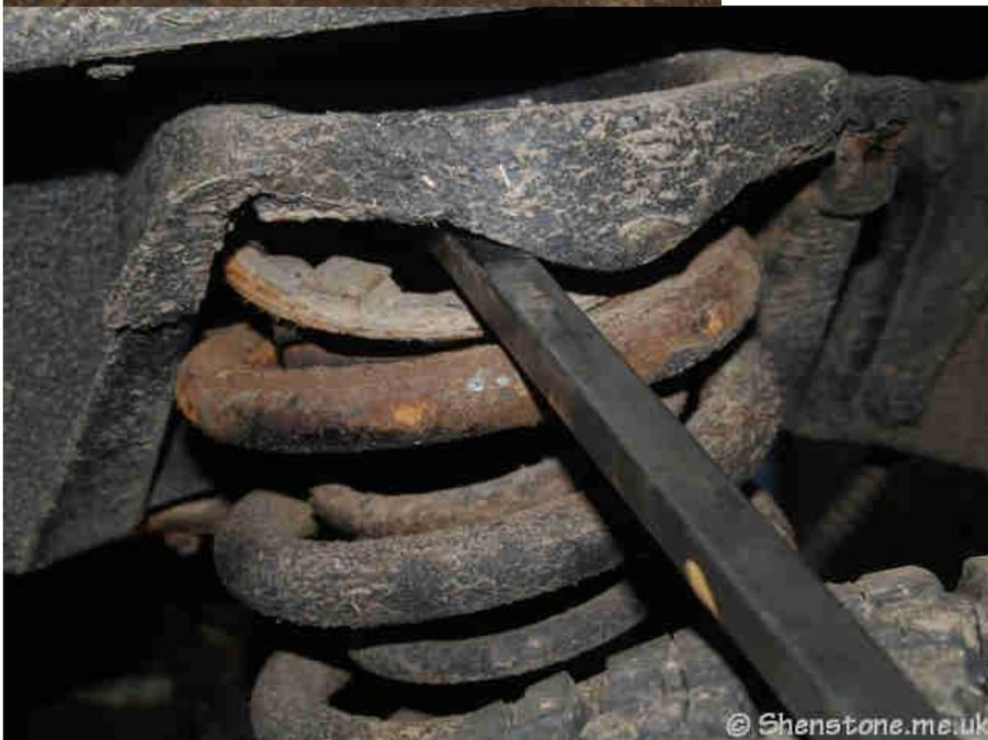
The spring was then levered out at the top with a tyre iron and the job went smoothly without the need for a jack to provide pressure
