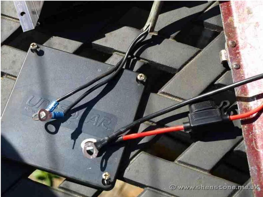
The new connections were all made in a waterproof housing which had grommets where the cable came through
