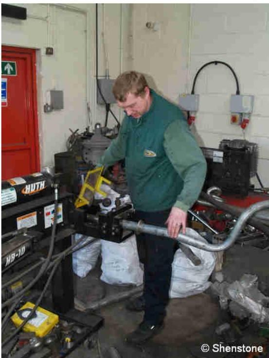
So this time it fitted first time, especially as I'd taken some more advice and lifted the chassis on a jack to give me more room over the rear axle. it reduced the stress in the job by about 95% Everything has of course been put back with new nuts and bolts where needed and lots of copper grease
