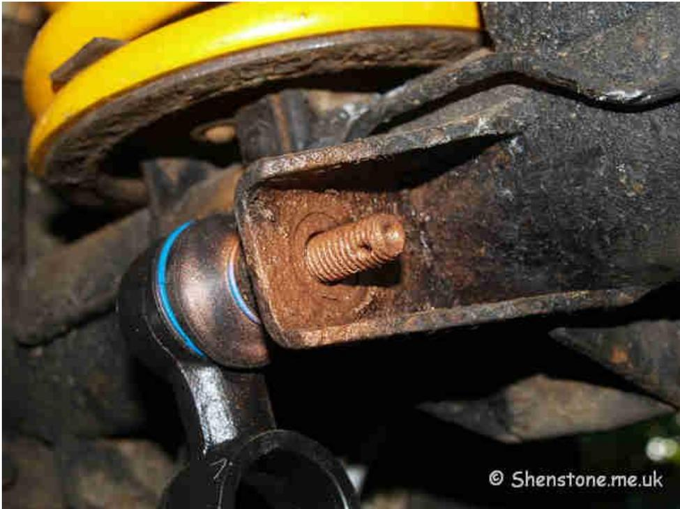
Putting the new one back with plenty of copper grease on the screw in case I ever need to remove it again
