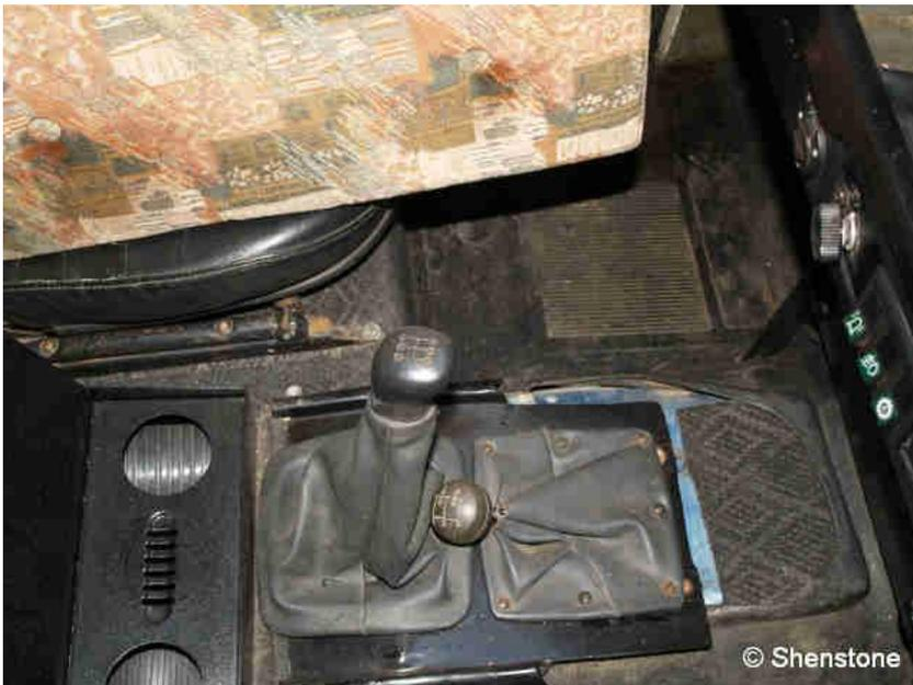
Then it was out with all the old and in with a load of sealant over all the gaps where panels were not fastened together well. Then, as with all jobs on Katy so far, nothing is entirely straightforward and the passenger side of the transmission tunnel was not fitted well to the foot well plates so the first thing we had to do was fix a strengthening plate across the screw fittings and seal up all the holes that could let water in.
