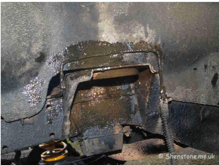
The new springs and shocks simply slotted into place and I had a spot of help from Dan who dropped by and showed me something I hadn't spotted (that the shock have a pair of flat sides at the top of the screw thread which you can put a set of mole grips or in this case a 9 mm spanner on. If you look back to the top of this post you can see them clearly, and realise what a dope I felt
