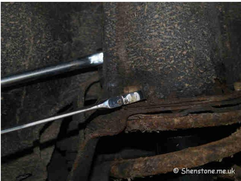
Removing the access panels in the engine bay to get at the top of the shock absorbers. In Katy this meant moving the coolant expansion tank first so I could get at one of them. The Drivers side came off easily, but the passenger side was well rusted on and it needed 2 of us (me holding on the flexible strap and Phil pulling on a long socket bar for leverage, but within a few minutes the old shocks and springs could be lifted out
