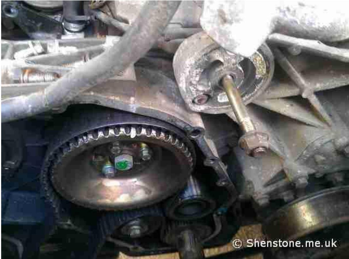
It was also noted that the bearing in the timing plate cover was rumbling and it would be a major cost and hassle if that failed and sent parts of the engine crashing into each other so that's been replaced as well
