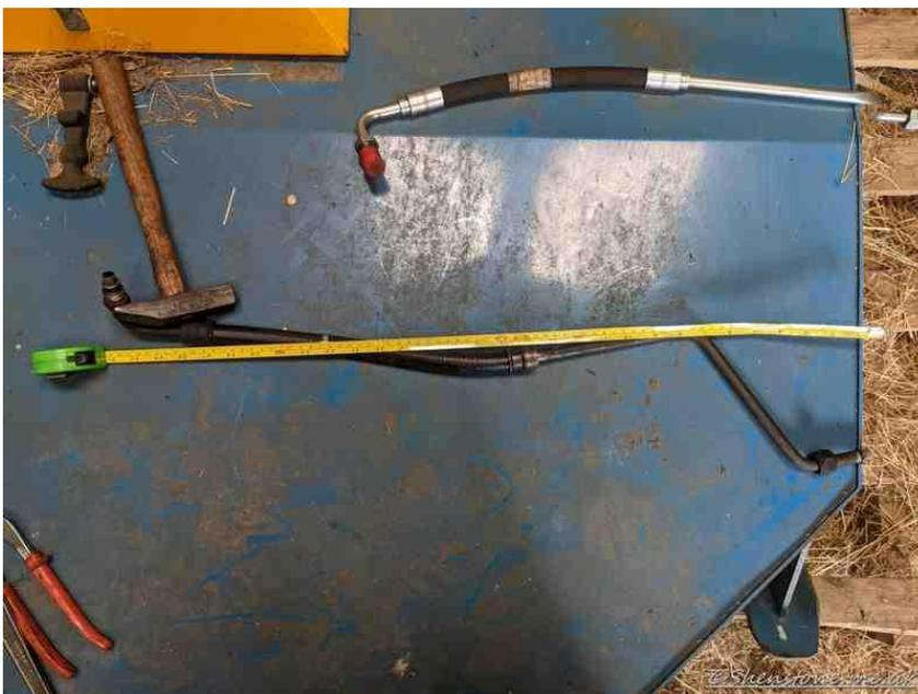
This is the old oil cooler pipe lined up with the edge of the machine
