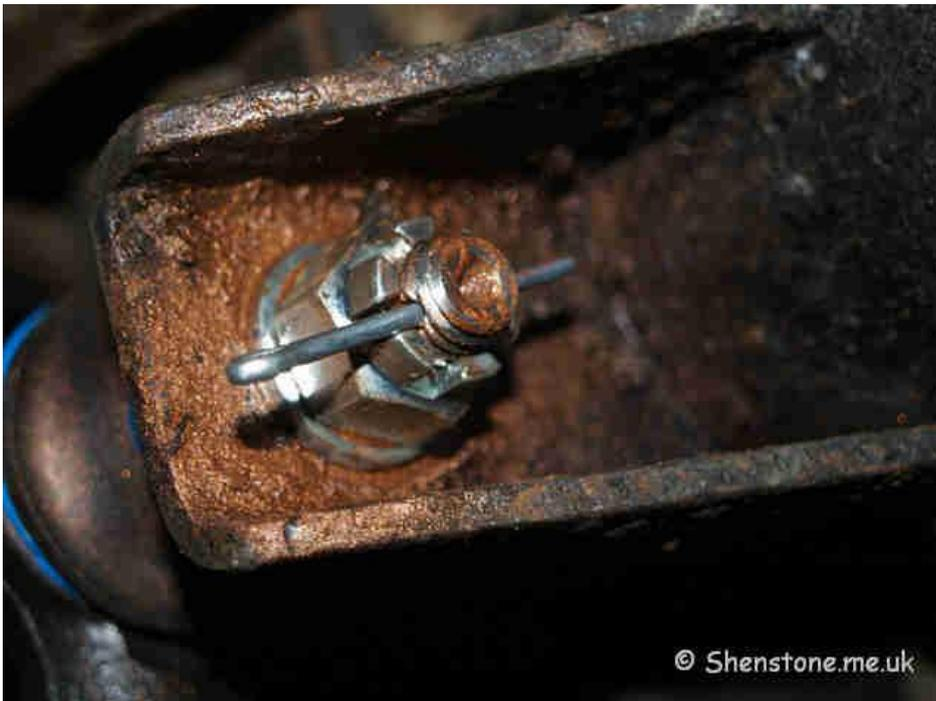
Then put the new bushes in place. The ones I had chosen were the blue polyurethane ones in the middle below. To be honest the old ones on the left and the new ones that came with the new linkages both looked OK, but everyone tells me the polyurethane ones will be stiffer and for £8.00 that's a good inexpensive addition that makes sense
