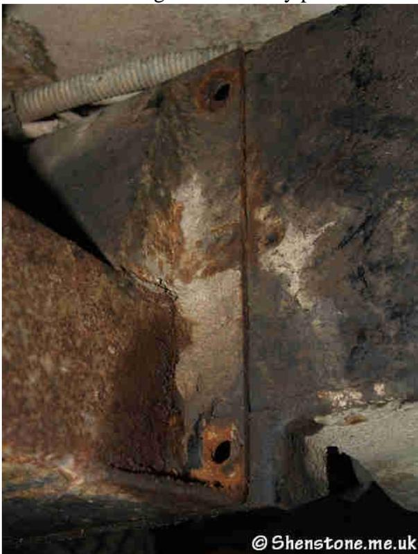
I struggled for ages trying to free up the handbrake to remove it and then Steve came back and showed me the correct bolts to undo which made the job a lot faster. The good news was that all of the clutch bell housing bolts came out easily (I was surprised) and then the whole gearbox came loose.
