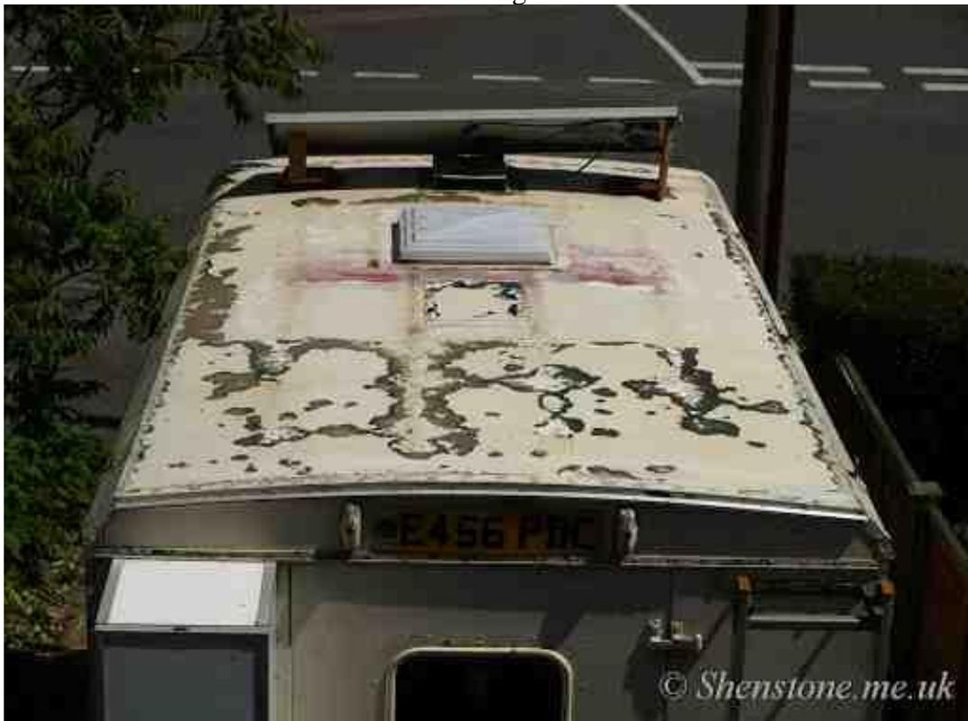
Much of the paint is so badly attached it comes in sheets with a scraper. this is not usual for automotive paint so I suspect that the final cream coat is more of a house paint than what is normally on a vehicle which is typically harder
