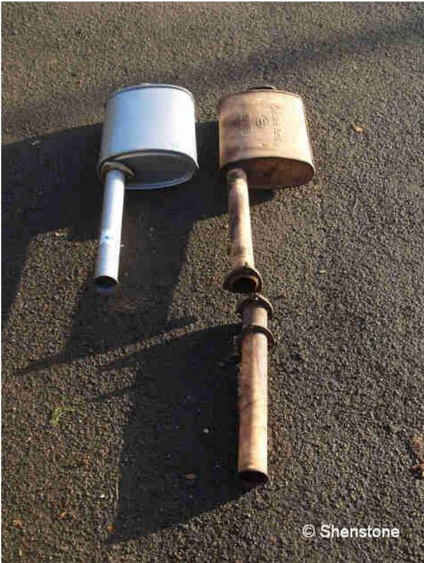
Here you can see the old and new center sections and the extra section that goes in a 110 Land Rover exhaust system in order to make it a 127 / 130 exhaust system. The sections are joined with the olive I referred to in a recent post
