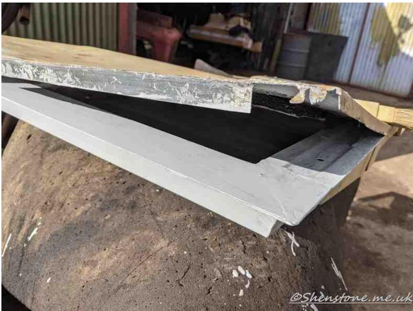
The door bottoms were rotten and were causing some bimetallic corrosion and the only way to resolve that is to peel open the door skin, clean up pretty much everything. put in new door frame
